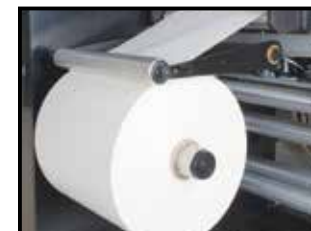
Pneumatically Activated Top Rider Rolls for Unsupported Film and Large Diameter Rewinding
