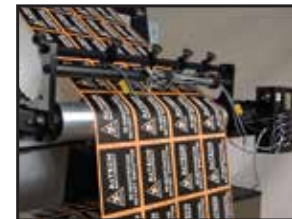
Electronic Missing Label, Splice and Flag Detection
